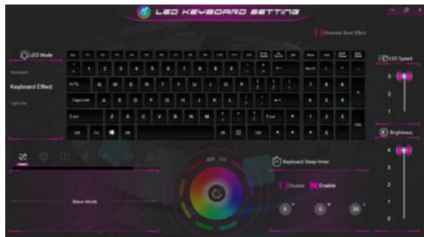
On boot the keyboard will momentarily flash. You can click in the **Override Boot Effect** check box to disable the keyboard flashing effect as the system boots.
